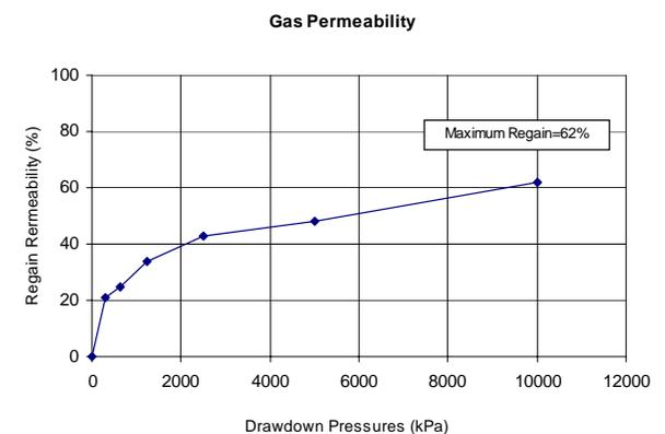
As illustrated by Figure #1, the drilling fluid invasion into the core plug of the untreated mud was 3.3 cm and a maximum permeability regain of 62% was achieved with a 10,000 KPa drawdown pressure.
